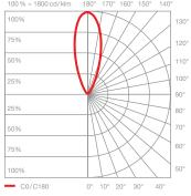
$\begin{array}{l} \textbf{uplight} \\ \text{direct, glare-free uplight (Occhio fireball optic),} \\ \text{beam angle approx. } 50^{\circ} \end{array}$
